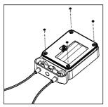
Mount the back cover. Place all five O-rings delivered with the battery.
