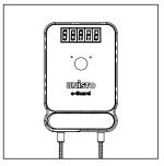
After that the display shows StArt for a short time. Now the seal is ready and creates sealing numbers.
