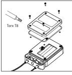
Remove the back cover and the old battey. Use a replacement battery from Unisto
