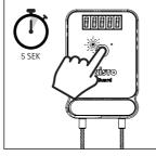
Activate and deactivate Bluetooth Touch the button for 5 seconds and the green LED starts/stops flashing.
