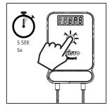
**Operations (oPS)** Touch the button 5-times in 5 seconds. The total amount of operations is shown.
