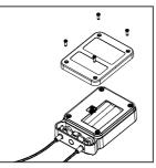
Fix the back plate with the four new screws. **Do not overtighten the** screws!
