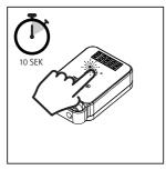
Push the touch button until the yellow LED flashes for the second time and the display shows "CAL". Push the button again and the display shows "oPEn". Push the button a second time and two different randomly generated 5 digit code appear on the display.
