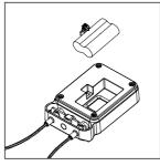
Plug in the new battery and turn the e-Guard to check the display.
