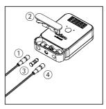
After the numbers "CLOSE" appears on the display and the new hasp ends must be inserted.
