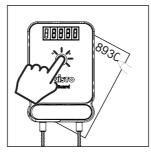
Push the button and write down the 4 digit unique sealing number.
