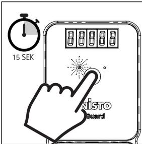
Press the touch for 15 seconds, when the green LED flashes for the 3rd time release the touch
